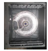
then lift out the filter plate (make sure to keep track of the O-ring underneath)
