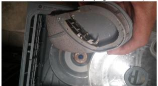
Clean the spray arm making sure to get all loose particles out of the inside
